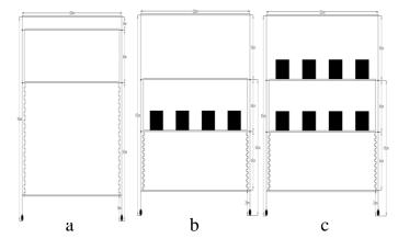
Figure 2: A graphical presentation of designed cart. a: empty, b:one shelf loaded, c: two shelves loaded
